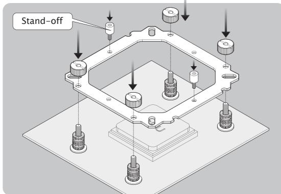
Then, aim the holes of mounting-clip to the Knurled threaded screws, then slip over the clips to the screw, and use metal nuts to fasten.
