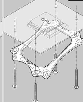
Aim the holes of back plate to the holes of MB, then let Knurled threaded screws through back plate and MB
