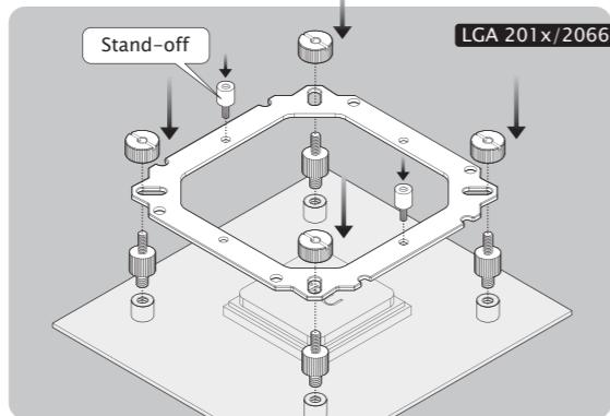
Fasten screws tightly onto MB. Aim the holes of Intel mounting-clip to the screws, and slip over the clips to the screw. Then, fasten the metal nuts onto screws.
