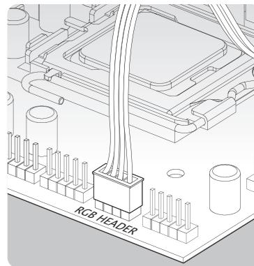
Use connect cable to link M/B RGB header.
