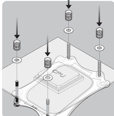
Use metal nuts to fasten back plate and MB
